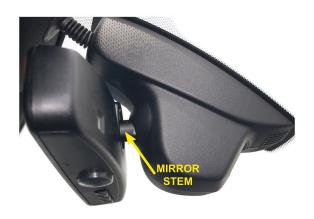
5 - While sitting in the passenger seat, place the mount over the mirror stem. Tighten the CLAMP SCREW until the mount starts to clamp onto the mirror stem. Position the mount as far forward as it will go and paralell to the bottom of the mirror before fully tightening.
