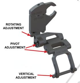
7 - Reinstall the body assembly. Be sure to include all lock washers with screws, and the lock and flat washer with the bottom socket head screw as shown above. Use the adjustments shown above to adjust the RD to your desired position. We recommend adjusting the RD as close to the bottom of mirror as possible. Be sure to tighten all screws after adjustments are made.
